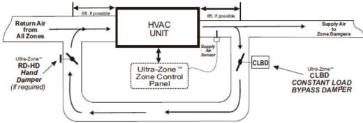
**Note:** This Drawing of the Bypass Damper, Balancing Hand Damper, and Related duct work is intended to serve only as a guide. Your actual duct work layout and components may differ. Use the graphic as a guide when planning or designing a Zone system regardless of Equipment type, Duct layout and Airflow configuration.
