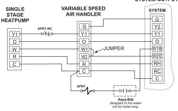
AFR1 - Model R1 SPDT Relay with 24 VAC Coil.
