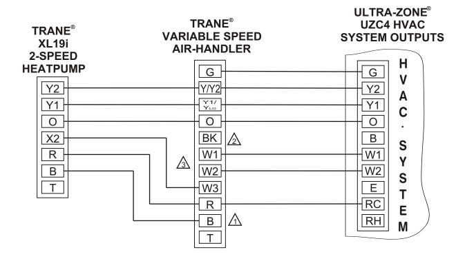
DO NOT CONNECT EQUIPMENT 24vac COMMON 'B' TERMINAL TO UZC4 PANEL
