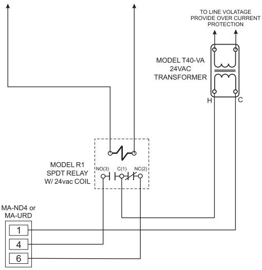
\*DAMPER WILL OPEN TO BRING IN FRESH AIR / COMBUSTION AIR WHEN COOLING IS ACTIVATED.
