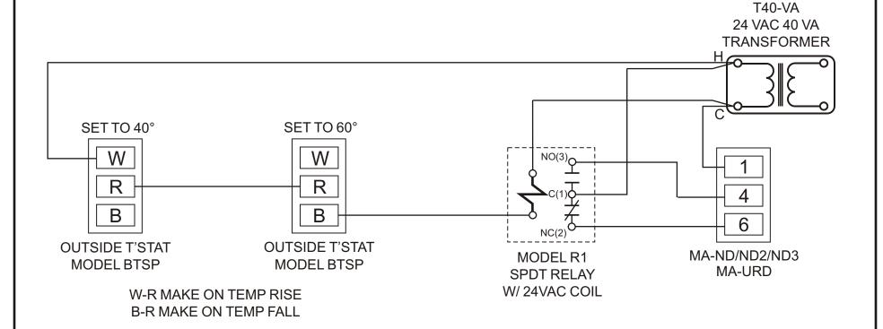
\*DAMPER WILL OPEN TO BRING IN FRESH AIR WHEN OUTSIDE TEMPERATURE IS BETWEEN 40° AND 60°
