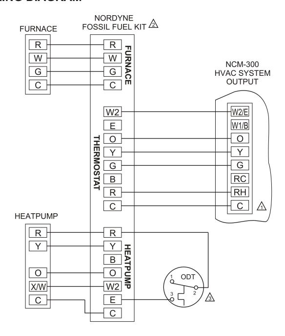
riangle OLDER VERSIONS OF THE NCM-300 DO NOT HAVE A 'C' TERMINAL ON THE SYSTEM TERMINAL BLOCK. DO NOT MAKE THIS CONNECTION IF NO 'C' TERMINAL IS PRESENT.
