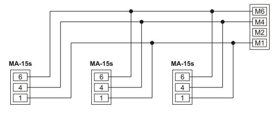
**NOTE:** You may electrically parallel several MA-15S motors together on a single zone. However, DO NOT parallel the EWC MA-15S with original Carrier/Bryant damper motors on the same zone. The back-feed characteristic of the Carrier/Bryant motors is not compatible with the MA-15S motors.
