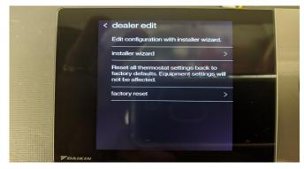
**Step 1:** Using the Daikin ONE+ thermostat connected to Zone 1 only, navigate to "**Dealer Edit**", insert the password and select the *Installer Wizard.*
