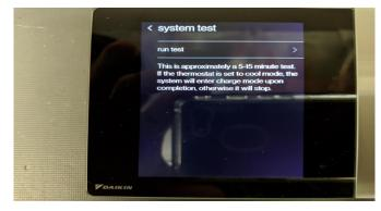
Step 6: Select the arrow and your Inverter Heat Pump or Air Conditioner test will start. The arrow will change to a spinning wheel indicating the test is underway. The test will last approx. 5 - 15 minutes. **DO NOT interrupt** *the test.*
