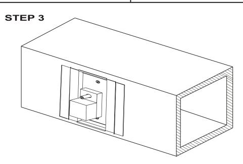
Insert the damper and put in the four corner screws. To secure the damper to the duct board.
