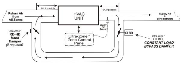
Note: This drawing of the Bypass damper, Balancing Hand Damper, and Related duct work is intended to serve only as a guide. Your actual duct work layout and components may differ. Use the graphic as a guide when planning or designing a Zone system regardless of the Equipment type, Duct layout and Airflow configuration.
