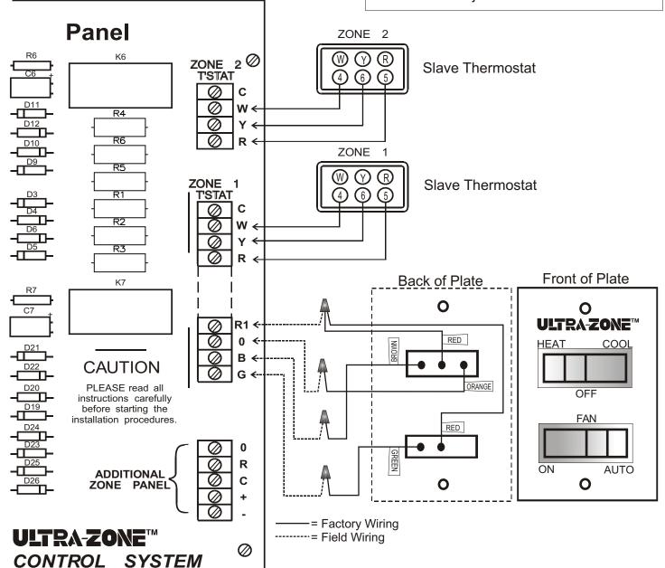
Follow the color coded wiring diagram to achieve manual changeover control of the HVAC system from Heating mode to Cooling mode. You can also achieve manual control of the system Fan operation. *Use 24vac only. Follow national and local electrical codes and ordinances.*
