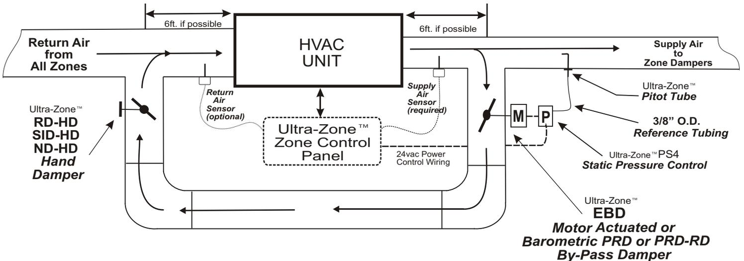
*Note: This EWC Controls drawing of the Bypass damper, Hand Damper, Static Pressure control and Related duct-work is intended to serve only as a guide. Your actual duct-work layout and components may differ. Use the graphic as a guide when planning or designing a Zone system regardless of the Equipment type, Duct layout and Airflow configuration.*
