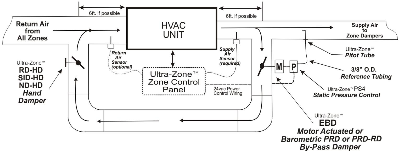
Note: This EWC Controls drawing of the Bypass damper, Hand Damper, Static Pressure control and Related duct-work is intended to serve only as a guide. Your actual duct-work layout and components may differ. Use the graphic as a guide when planning or designing a Zone system regardless of the Equipment type, Duct layout and Airflow configuration.
